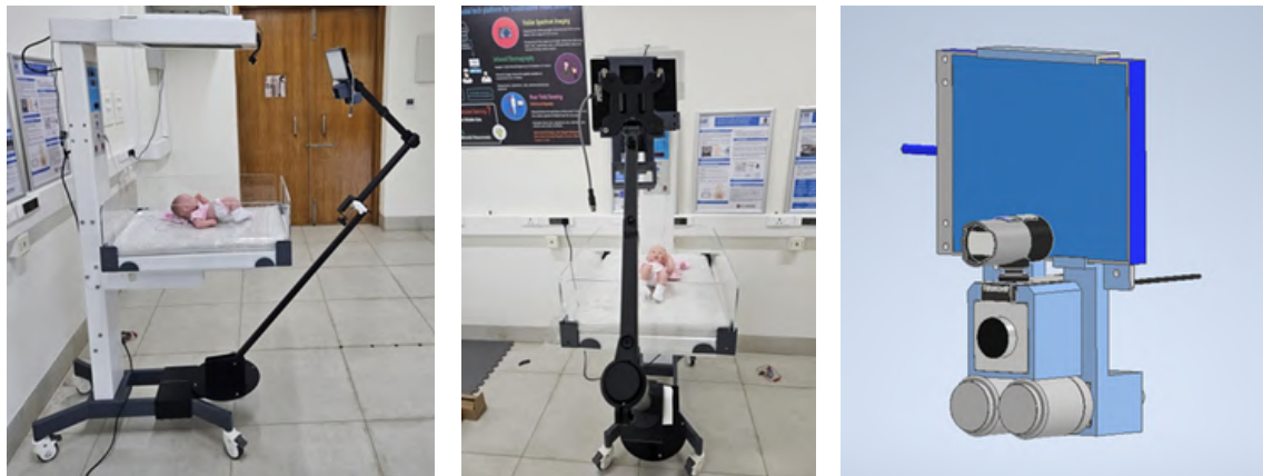
Fig. 2: Rotatable non-contact data-collection set-up designed for monitoring on a radiant warmer. The measurement setup can be moved around to make way for care-giver access. The setup consists of four different cameras
