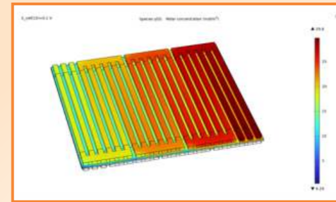
Oxygen molar concentration (mol/m 3 ) at the cathode side of PEM fuel cell
