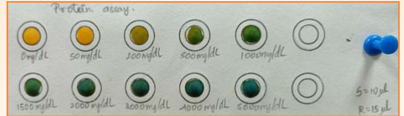
Protein Standard Assay in Paper Microfluidic device
