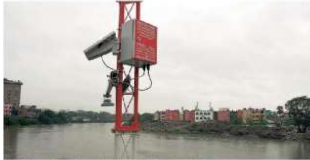
Crucial inputs: A flood sensor installed at Saidapet by IIT-Madras. •R. PICHUMAN
