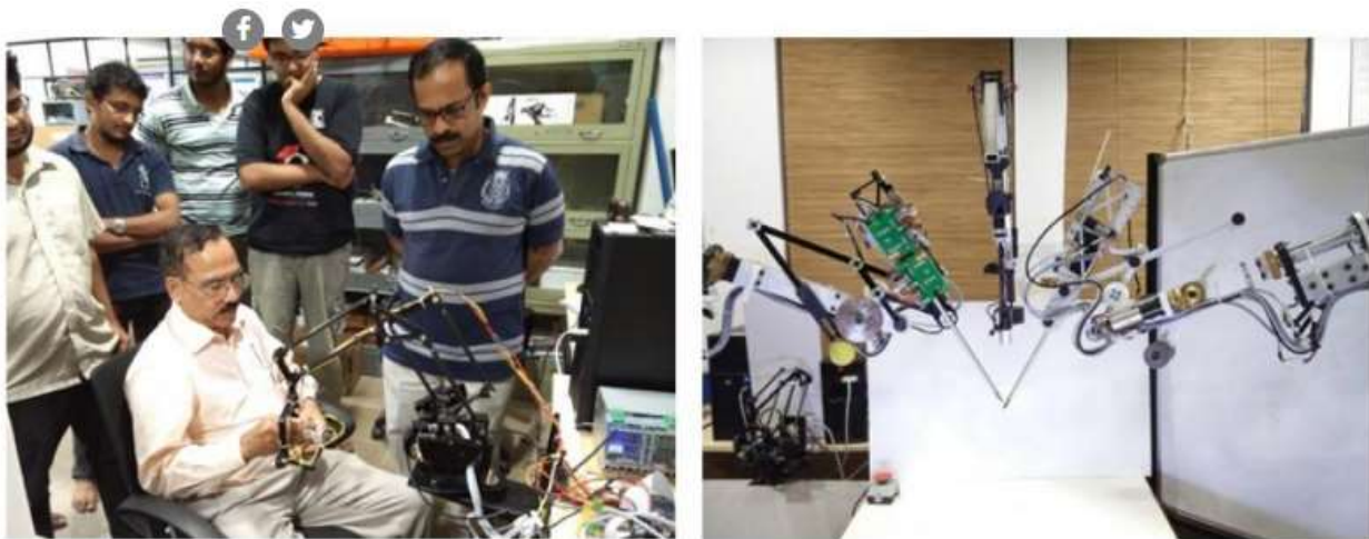
📷 IIT-M team with its trainer robot (left) and slave arms of the robot (right). Credit: India Science Wire
