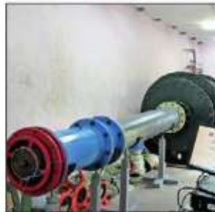
WAVE ENERGY: The 'impulse' turbine works with a unidirectional rotor powered by a generator
