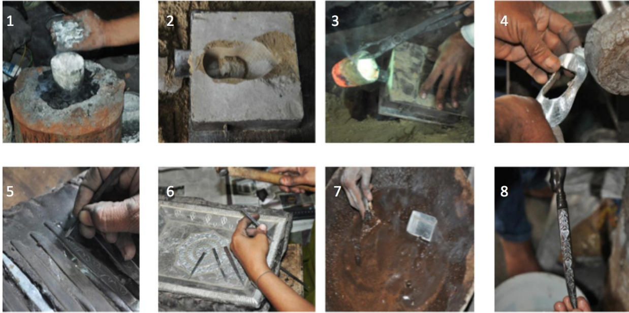
FIGURE 1.2: Steps of Manufacturing of Bidriware craft (1-Melting, 2-Moulding, 3-Pouring, 4-Machining, 5-Pattern Etching, 6-Engraving, 7-Patination, 8-Final product [16])
