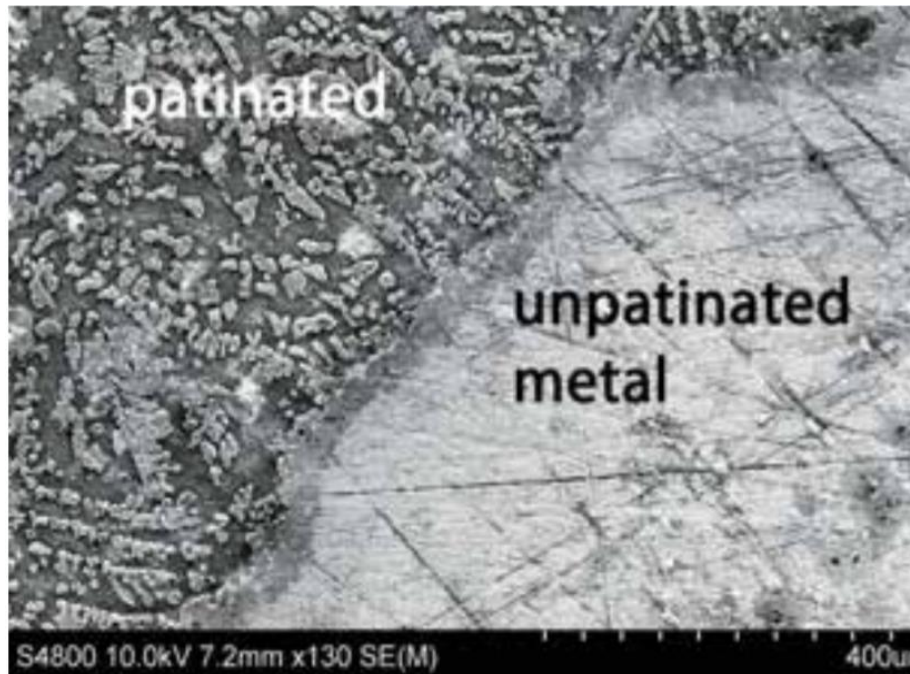
FIGURE 2.2:- SEM secondary electron image of a part-patinated piece of experimental bidri alloy. [3]
