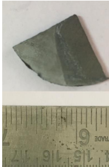
FIGURE 5.16: Specimen subjected to alternative process-4 solution that contains 1:20 weight ratio of \text{KNO}_3 and \text{NH}_4\text{Cl} in De-ionised water for 24 seconds
